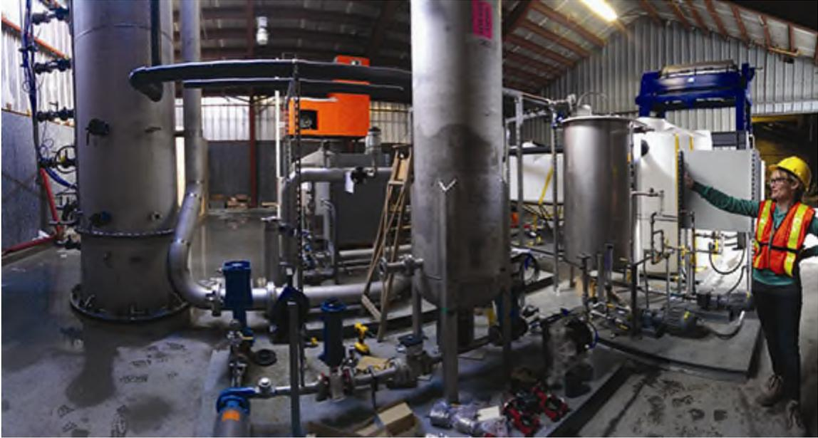
The technology start-up is putting up money to prove its concept. At Squamish, in British Columbia, Canada, CE has built a pilot plant capable of capturing 500 tonnes/year of CO<sub>2</sub> and is setting about capturing operational data that will enable it to scale up to commercial size of around 1m tonnes/year – equivalent, it says, to taking 250,000 cars off the road. The move towards a full-scale plant should be possible in 2017, says the company.
